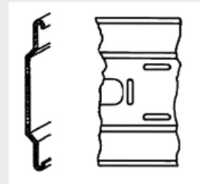
Profile and top view of the 86.5 mm profile rail.
